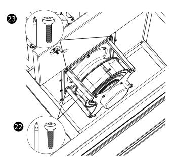
To replace the fan assembly, locate the mounting plate over the fixings retained in the unit bulkhead. Secure the loose fixings through the mounting plate and tighten all the mounting fixings. Reconnect the supply plugs as in Fig. (2); if more than one plug is used, ensure the correct plugs are reconnected as marked. Ensure that the fans are free running by following the fan alignment instructions in Fig. (2) on page 13, adjust as required.
