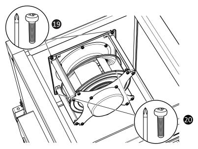
To replace the fan assembly, locate the mounting plate over the fixings retained in the unit bulkhead. Secure the loose fixings through the mounting plate and tighten all the mounting fixings. Reconnect the supply plugs as in Fig. 22; if more than one plug is used, ensure the correct plugs are reconnected as marked. Ensure that the fans are free running by following the fan alignment instructions in Fig. 21, adjust as required.
