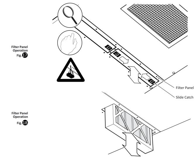
To replace, dispose of the old filters responsibly, note the airflow direction arrow on the new filter. Slide the clean filter into the unit and replace the filter doors.
