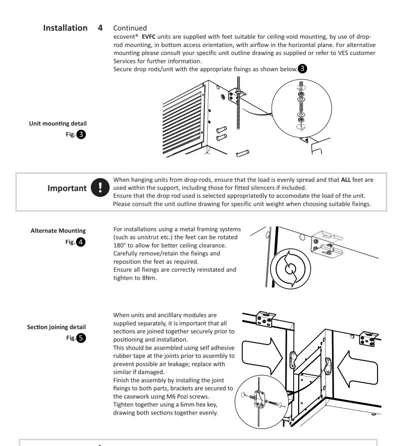
Joining brackets are **NOT** structural and are included as part of the unit sealing only. When moving assembled units ensure that **ALL** sections are fully supported.
