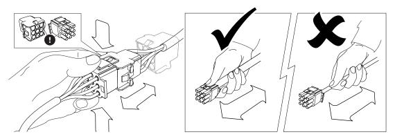
On reconnection, the assembly features a locating lug to ensure correct orientation. Once rejoined, lock the connection together again using the system as shown. Note the plugs are handed and forcing an incorrect connection may result in damage to the plug.
