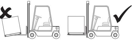
Handle with care. Failure to fully support the unit during lifting may result in damage to the unit.
