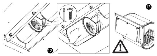
Extract Fan assembly removal/installation
